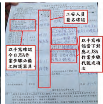
Example of JSA inspection
